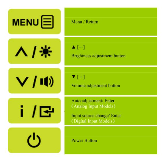
Figure.4. Control Panel Buttons
